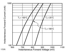
Figure 2. Typical Instantaneous Forward Characteristics
