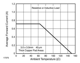
Figure 1. Forward Current Derating Curve
