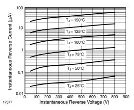
Figure 3. Typical Instantaneous Reverse Characteristics
