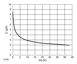
Figure 4. Capacitance vs. Reverse Voltage
