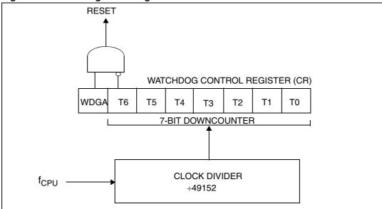
Figure 23. Watchdog block diagram
