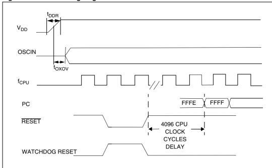
Figure 12. Reset timing diagram
