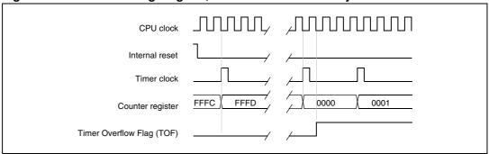
Figure 28. Counter timing diagram, internal clock divided by 8
