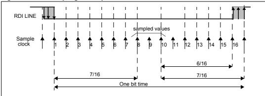
Figure 40. Bit sampling in reception mode
