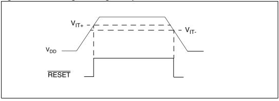
Note: Hysteresis  $(V_{IT+}-V_{IT-}) = V_{hys}$
