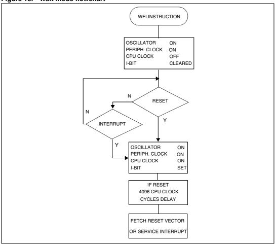
Note: Before servicing an interrupt, the CC register is pushed on the stack. The I-Bit is set during the interrupt routine and cleared when the CC register is popped.
