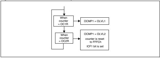
If OLVL1 = 1 and OLVL2 = 0, the length of the positive pulse is the difference between the OC2R and OC1R registers.
