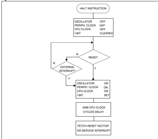
Figure 17. Halt mode flowchart
