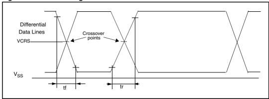
Figure 66. USB: data signal rise and fall time
