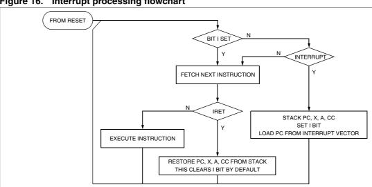
Figure 16. Interrupt processing flowchart
