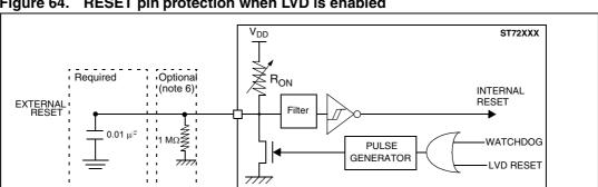
Figure 64. RESET pin protection when LVD is enabled
