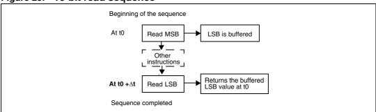
The user must first read the MSB, afterwhich the LSB value is automatically buffered.
