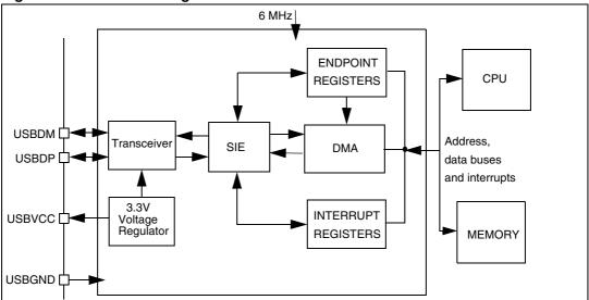
Figure 41. USB block diagram
