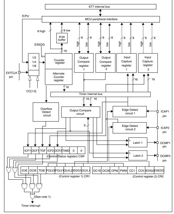
Figure 24. Timer block diagram
