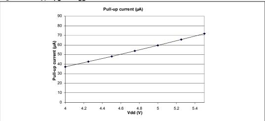
Figure 53. Typ.  $R_{PU}$  vs.  $V_{DD}$
