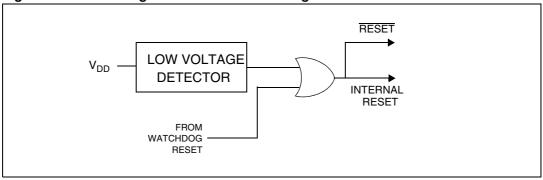
Figure 10. Low voltage reset signal output
