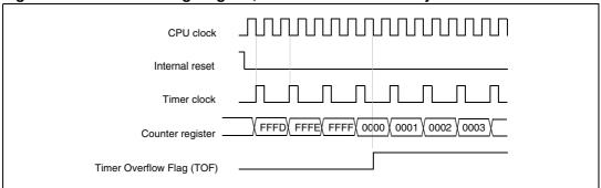
Figure 27. Counter timing diagram, internal clock divided by 4
