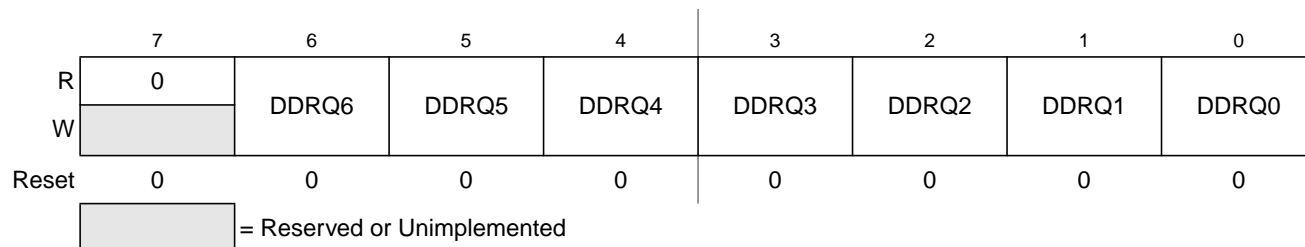
Figure 3-25. Port Q Data Direction Register (DDRQ)
