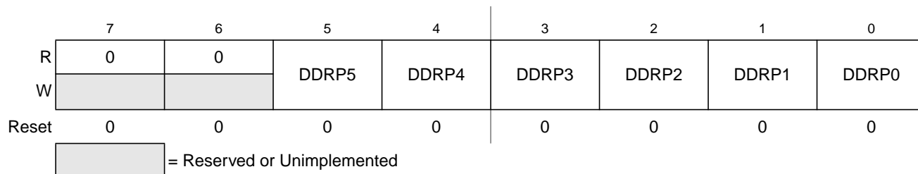
Figure 3-19. Port P Data Direction Register (DDRP)
