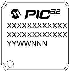
100-Lead TQFP (14x14x1 mm)
