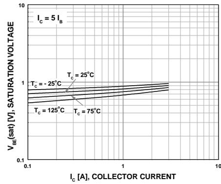
Figure 4. Saturation Voltage
