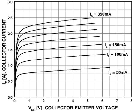
Figure 1. Static Characteristic
