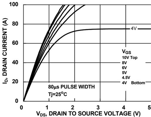
Figure 9. Saturation Characteristics
