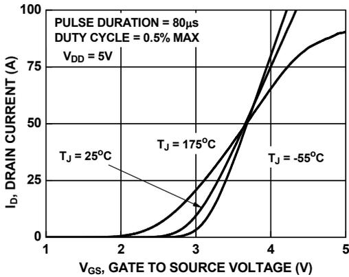
Figure 7. Transfer Characteristics
