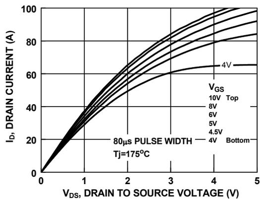
Figure 10. Saturation Characteristics
