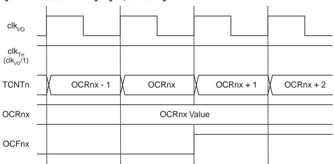
Figure 48. Timer/Counter Timing Diagram, no Prescaling
