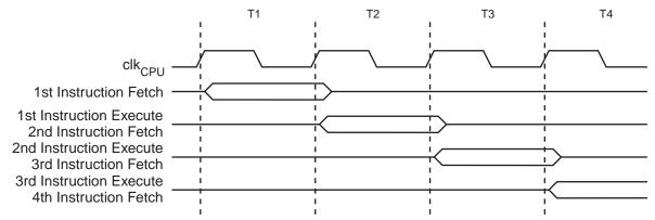
Figure 8 shows the internal timing concept for the Register File. In a single clock cycle an ALU operation using two register operands is executed, and the result is stored back to the destination register.
