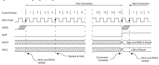
Figure 57. ADC Timing Diagram, Single Conversion
