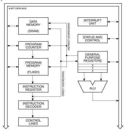
In order to maximize performance and parallelism, the AVR uses a Harvard architecture – with separate memories and buses for program and data. Instructions in the Program memory are executed with a single level pipelining. While one instruction is being executed, the next instruction is pre-fetched from the Program memory. This concept enables instructions to be executed in every clock cycle. The Program memory is In-System Reprogrammable Flash memory.
