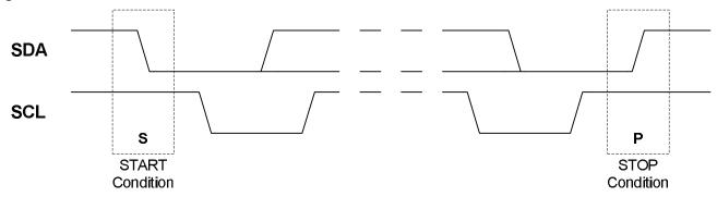
Multiple START conditions can be issued during a single transaction. A START condition not directly following a STOP condition, are named a Repeated START condition (Sr).
