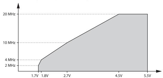
Figure 101. Maximum Operating Frequency vs. Supply Voltage
