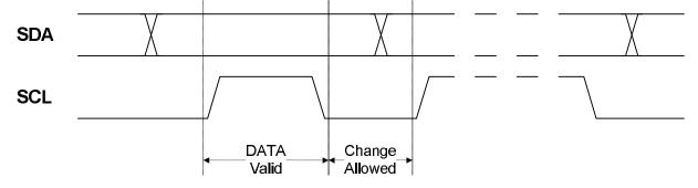
Combining bit transfers results in the formation of address and data packets. These packets consist of 8 data bits (one byte) with the most significant bit transferred first, plus a single bit not-acknowledge (NACK) or acknowledge (ACK) response. The addressed device signals ACK by pulling the SCL line low, and NACK by leaving the line SCL high during the ninth clock cycle.
