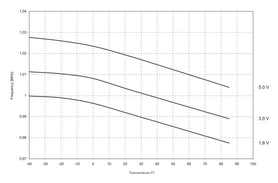
Figure 181. Calibrated Oscillator Frequency vs. Temperature (Two-point Calibration)
