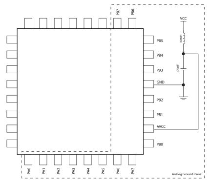
Where high ADC accuracy is required it is recommended to use ADC Noise Reduction Mode, as described in Section 15.7 on page 144. This is especially the case when system clock frequency is above 1 MHz, or when the ADC is used for reading the internal temperature sensor, as described in Section 15.12 on page 148. A good system design with properly placed, external bypass capacitors does reduce the need for using ADC Noise Reduction Mode
