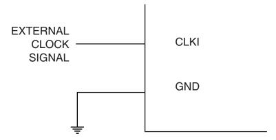
Start-up time for this clock source is determined by the SUT fuse bit, as shown in Table 7 on page 30.
