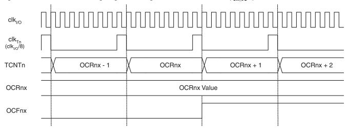
Figure 36 on page 97 shows the setting of OCF0A and the clearing of TCNT0 in CTC mode and fast PWM mode where OCR0A is TOP.
