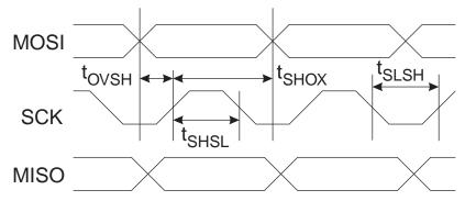
Figure 108. Serial Programming Waveform
