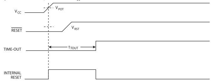
Figure 15. MCU Start-up, RESET Extended Externally
