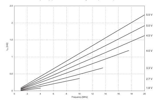
Figure 123. Reset Current vs. V<sub>CC</sub> (No Clock, excluding Reset Pull-Up Current)
