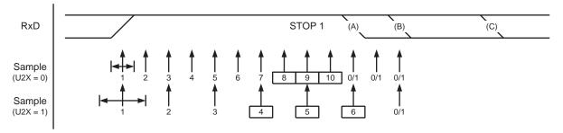
The stop bit is subject to the same majority voting as the other bits in the frame. If the stop bit is registered to have a logic low value, the Frame Error flag (FE) will be set.
