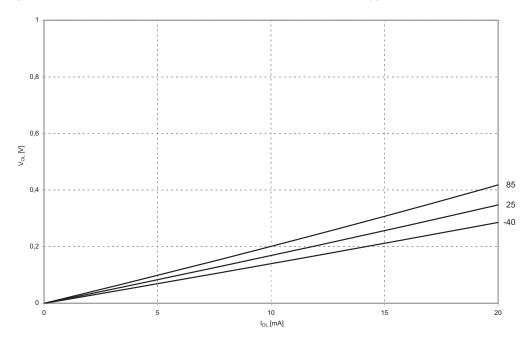
Figure 161.  $V_{OL}$ : Output Voltage vs. Sink Current (Extra High Sink I/O Pin,  $V_{CC} = 5V$ )
