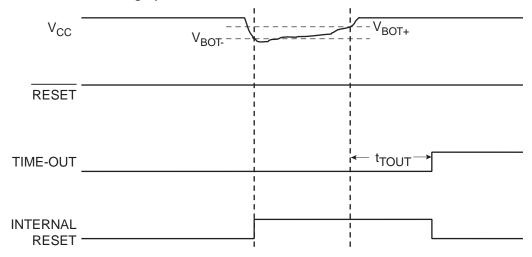
The BOD circuit will not detect a drop in  $V_{CC}$  unless the voltage stays below the trigger level for the detection time,  $t_{BOD}$  (see "System and Reset Characteristics" on page 250).
