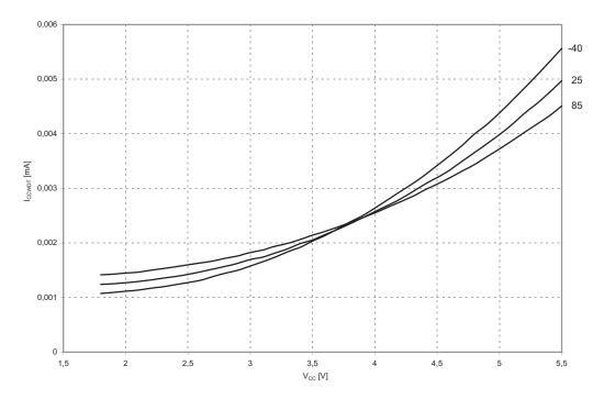
Figure 127. Brownout Detector Current vs.  $V_{\text{CC}}$
