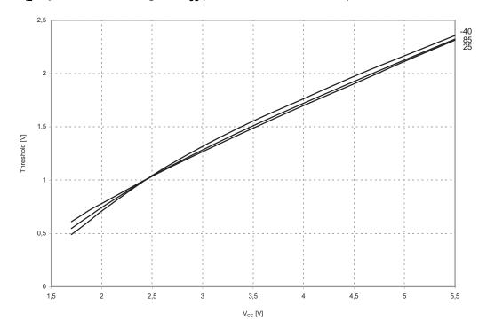
Figure 143.  $V_{IH}$ - $V_{IL}$ : Input Hysteresis vs.  $V_{CC}$  (Reset Pin as I/O)
