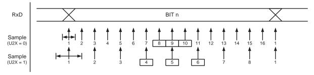
The decision of the logic level of the received bit is taken by doing a majority voting of the logic value to the three samples in the center of the received bit. In the figure, the center samples are emphasized by having the sample number inside
