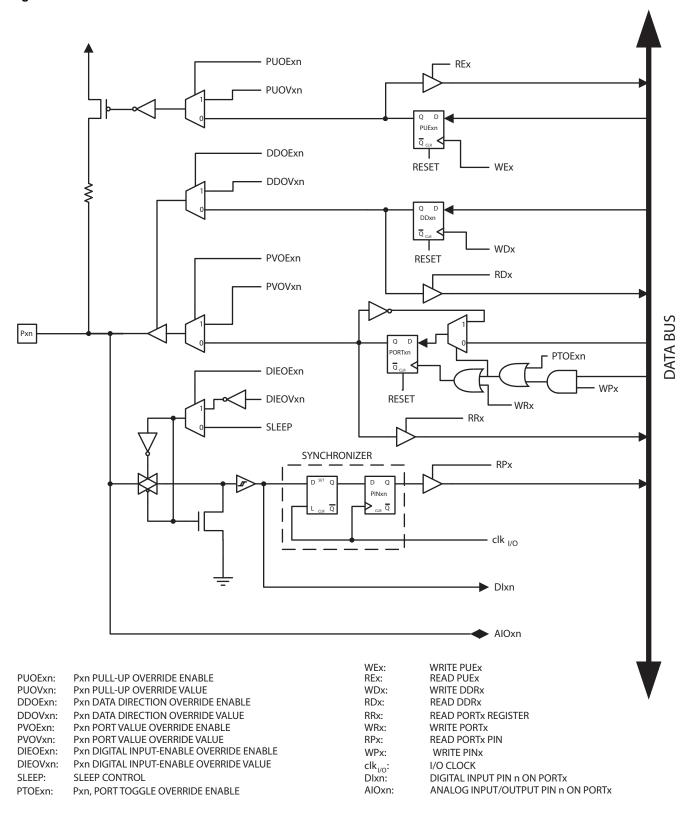
Note: WEx, WRx, WPx, WDx, REx, RRx, RPx, and RDx are common to all pins within the same port. clk<sub>I/O</sub>, and SLEEP are common to all ports. All other signals are unique for each pin.
