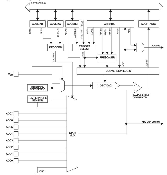
Figure 53. Analog to Digital Converter Block Schematic
