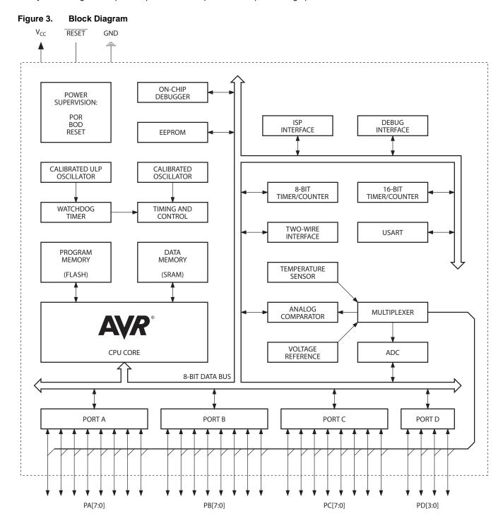
The AVR core combines a rich instruction set with 32 general purpose working registers. All 32 registers are directly connected to the Arithmetic Logic Unit (ALU), allowing two independent registers to be accessed in a single instruction, executed in one clock cycle. The resulting architecture is compact and code efficient while achieving throughputs up to ten times faster than conventional CISC microcontrollers.
