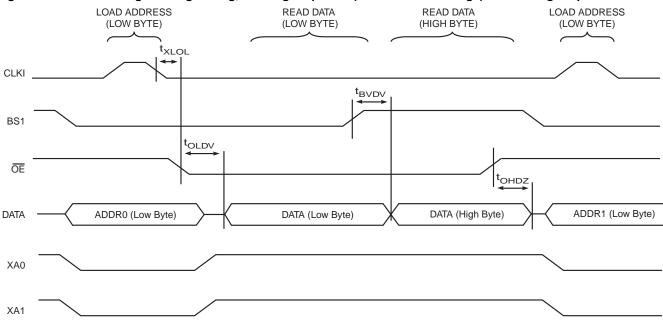
Note: 1. The timing requirements shown in Figure 104 (i.e.,  $t_{DVXH}$ ,  $t_{XHXL}$ , and  $t_{XLDX}$ ) also apply to reading operation.
