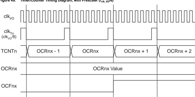
Figure 49. Timer/Counter Timing Diagram, with Prescaler (f<sub>clk I/O</sub>/8)
