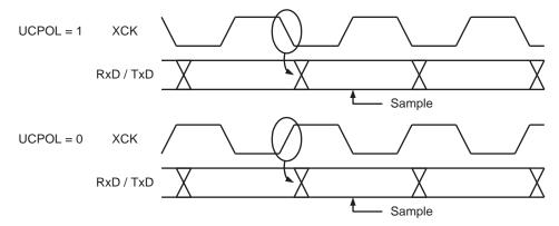
As shown in Figure 72, when UCPOL is set, the data is changed at falling XCK edge and sampled at rising XCK edge. When UCPOL is cleared, the data is changed at rising XCK edge and sampled at falling XCK edge.
