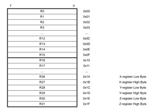
Most of the instructions operating on the Register File are single cycle instructions with direct access to all registers.
