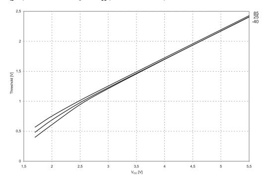
Figure 137.  $V_{IH}$ - $V_{IL}$ : Input Hysteresis vs.  $V_{CC}$  (I/O Pin)
