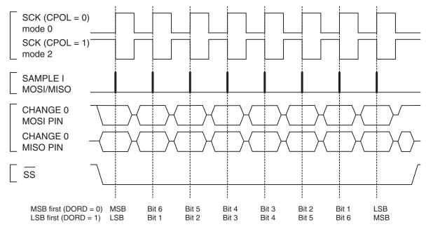
Figure 69. SPI Transfer Format with CPHA = 1
