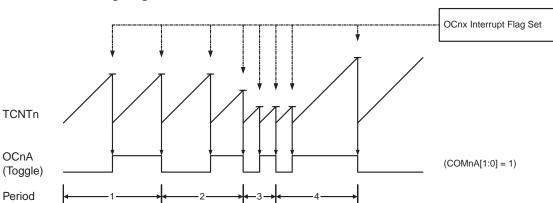
Figure 30. CTC Mode, Timing Diagram
