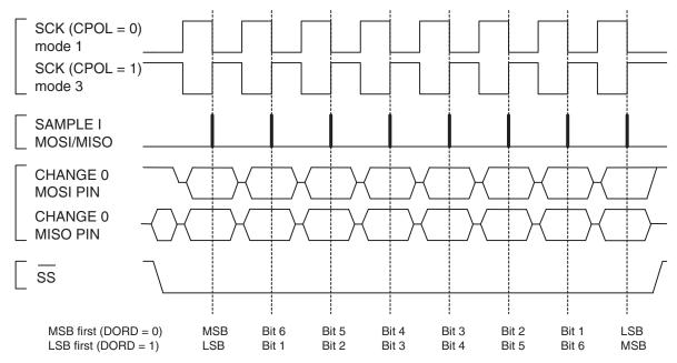
Data bits are shifted out and latched in on opposite edges of the SCK signal, ensuring sufficient time for data signals to stabilize. This is shown in Table 56, which is a summary of Table 57 on page 161 and Table 58 on page 162.
