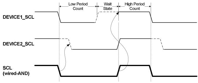
A high to low transition on the SCL line will force the line low for all masters on the bus and they start timing their low clock period. The timing length of the low clock period can vary between the masters. When a master (DEVICE1 in this
