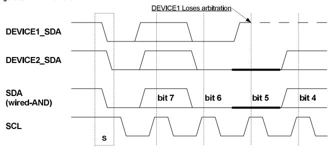
Figure 86 shows an example where two TWI masters are contending for bus ownership. Both devices are able to issue a START condition, but DEVICE1 loses arbitration when attempting to transmit a high level (bit 5) while DEVICE2 is transmitting a low level.
