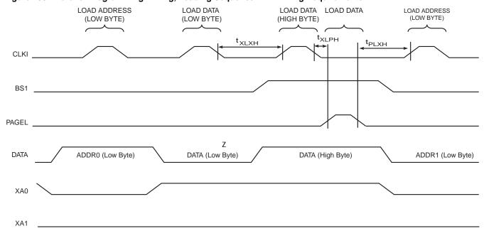
Note: 1. The timing requirements shown in Figure 104 (i.e.,  $t_{DVXH}$ ,  $t_{XHXL}$ , and  $t_{XLDX}$ ) also apply to loading operation.
