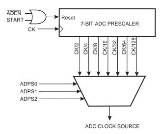
The ADC module contains a prescaler, as illustrated in Figure 55 on page 140, which generates an acceptable ADC clock frequency from any CPU frequency above 100 kHz. The prescaling is set by the ADPS bits in ADCSRA. The prescaler starts counting from the moment the ADC is switched on by setting the ADEN bit in ADCSRA. The prescaler keeps running for as long as the ADEN bit is set, and is continuously reset when ADEN is low.
