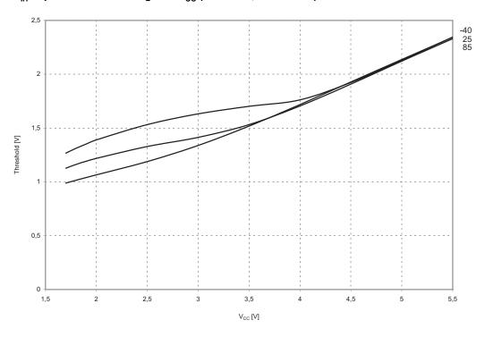
Figure 145.  $V_{IL}$ : Input Threshold Voltage vs.  $V_{CC}$  (Reset Pin, Read as '0')
