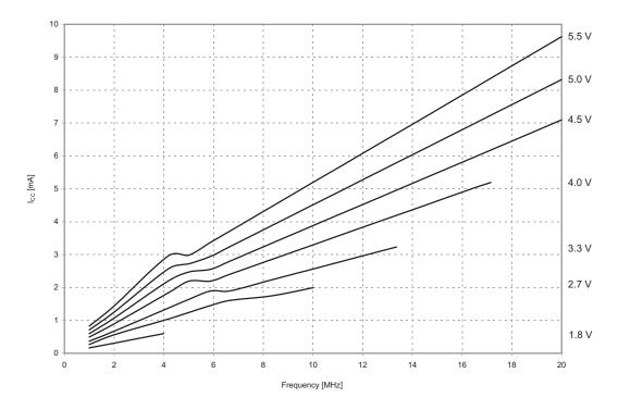
Figure 111. Active Supply Current vs.  $V_{\rm CC}$  (Internal Oscillator, 8 MHz)
