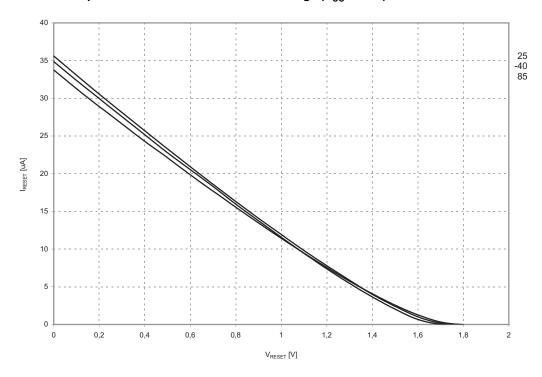
Figure 133. Reset Pull-up Resistor Current vs. Reset Pin Voltage ( $V_{CC} = 2.7V$ )
