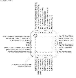
Figure 2. ATtiny828 Pinout in TQFP32.
