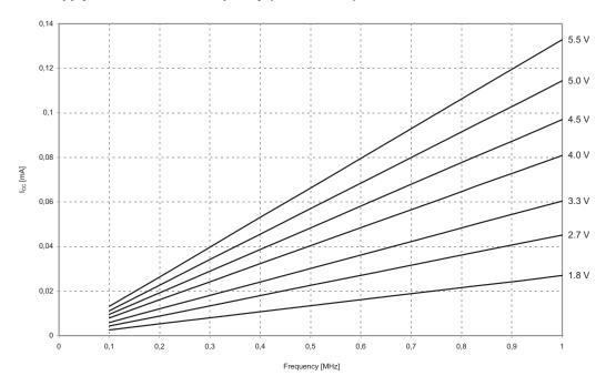
Figure 115. Idle Supply Current vs. Frequency (1 - 20 MHz)
