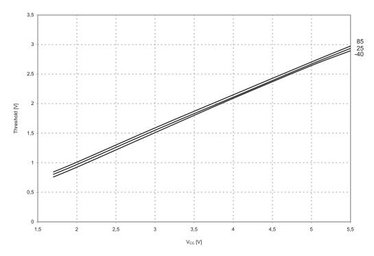
Figure 139.  $V_{\rm IL}$ : Input Threshold Voltage vs.  $V_{\rm CC}$  (I/O Pin, Read as '0')
