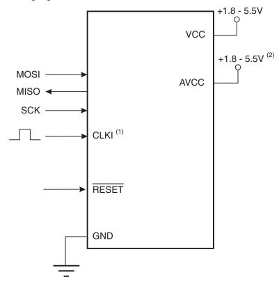
Notes: 1. If the device is clocked by the internal oscillator there is no need to connect a clock source to the CLKI pin.
