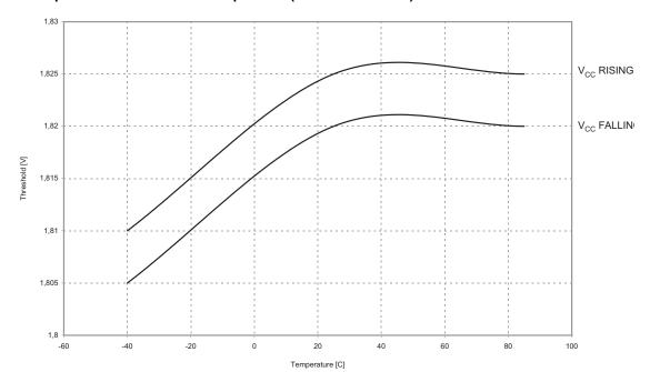
Figure 170. Sampled BOD Threshold vs Temperature (BODLEVEL = 1.8V)
