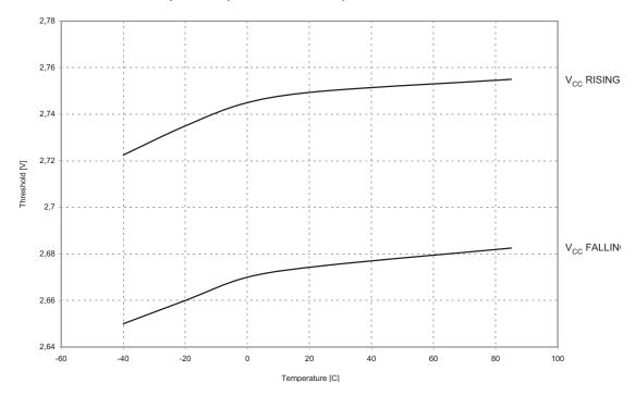
Figure 167. BOD Threshold vs Temperature (BODLEVEL = 1.8V)
