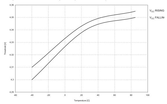
Figure 169. Sampled BOD Threshold vs Temperature (BODLEVEL = 2.7V)
