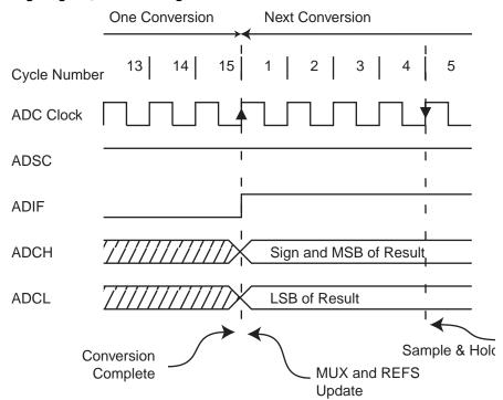
Figure 59. ADC Timing Diagram, Free Running Conversion
