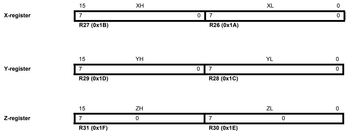
Figure 4-3. The X-, Y-, and Z-registers
