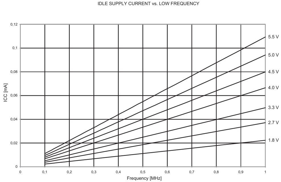
Figure 21-6. Idle Supply Current vs. Low Frequency (0.1 - 1.0 MHz)
