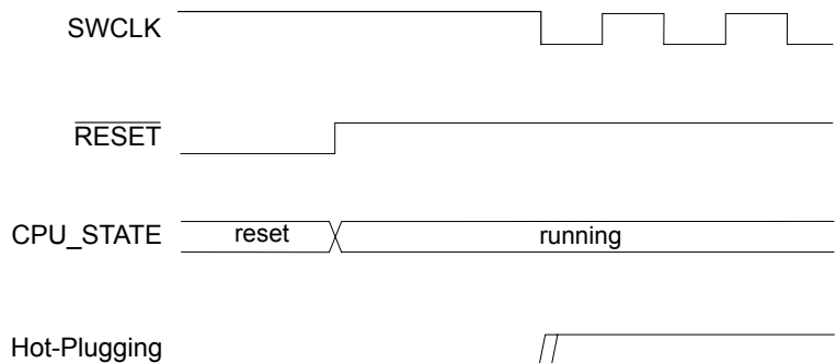
Figure 13-3. Hot-Plugging Detection Timing Diagram
