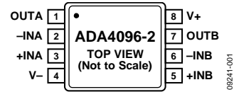
Figure 1. 8-Lead, MSOP (RM-8), ADA4096-2
