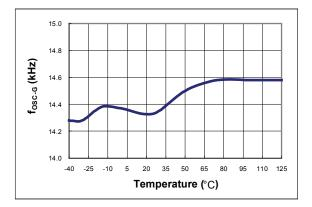
Figure 10. Green-Mode Frequency (f<sub>OSC-G</sub>) vs. Temperature
