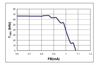
Figure 11. PWM Oscillator Frequency (f<sub>OSC</sub>)
