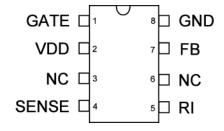
Figure 5. DIP-8 Pin Configuration
