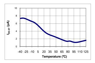
Figure 8. Startup Current (IDD-ST) vs. Temperature
