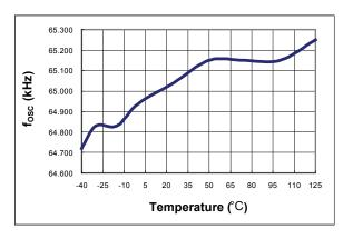
Figure 9. Center Frequency (fosc) vs. Temperature
