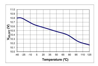
Figure 7. Turn-Off Threshold Voltage ( $V_{DD\text{-}OFF}$ ) vs. Temperature
